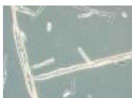
Fig. 2a: Microscopy picture of soda-AQ fibers in 10 times enlargement
